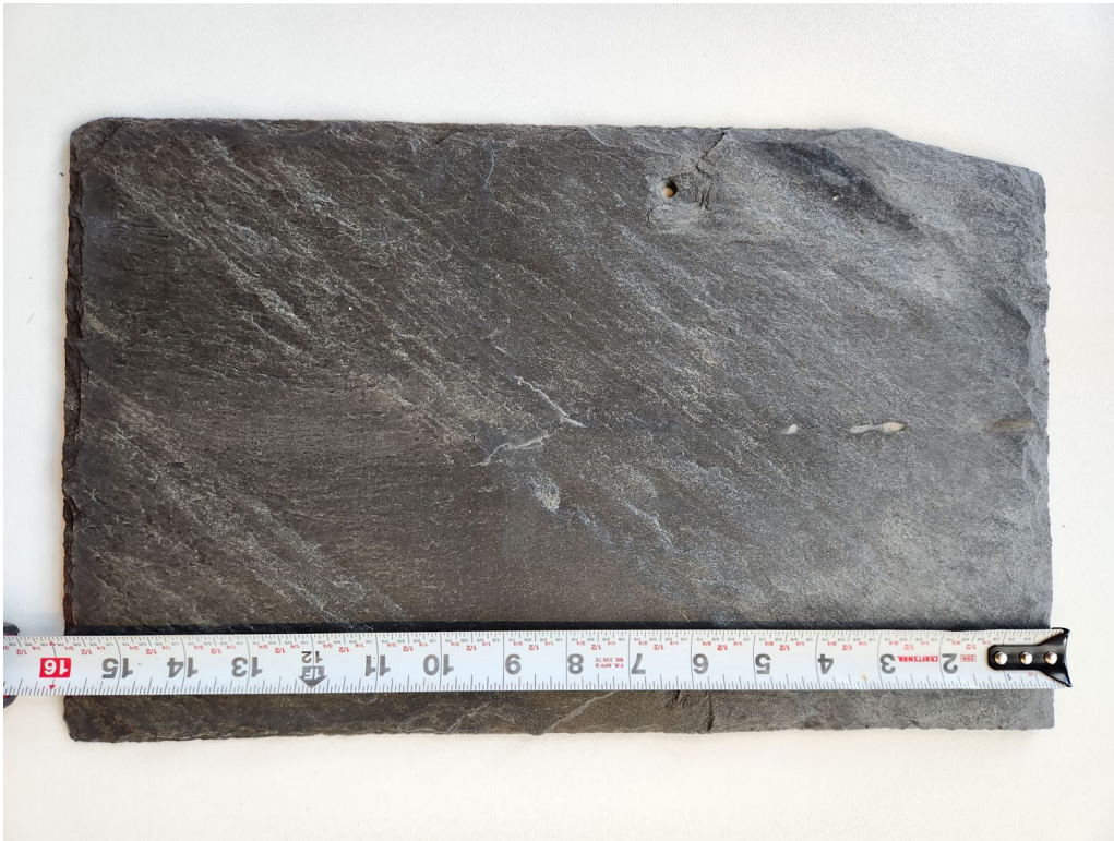
3. Salvaged historic Buckingham slate, typical condition
